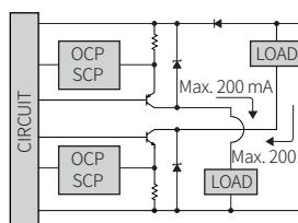
• OCP (over current protection, 过电流保护回路), SCP (short circuit protection, 短路保护回路)
